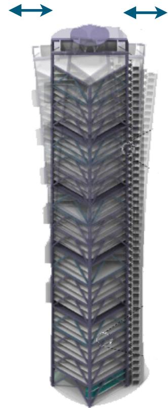
The structure is able to oscillate up to 2 meters at the top to release load.
